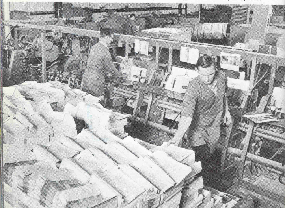
Above, one of the Miehle-Goss 4-color web-fed offset presses, Pasadena plant of Ambassador College Press. Below, one of two large McCain binderies — puts various signatures of magazines together, staples, binds, trims, turning out completed magazines at rapid speed.
